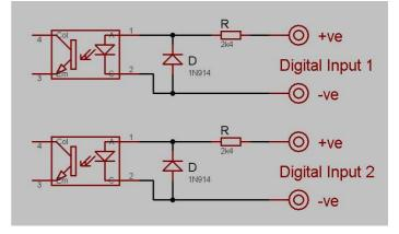
Thus to use a 48V power supply, an external resistor of ~2400 $\Omega$  is required (standard values of 2k2 $\Omega$  or 2k7 $\Omega$  would suffice); power dissipation would be (I<sup>2</sup>R) 0.01 \* 0.01 \* 2400 = 0.24W, so a standard 0.5W or 0.6W resistor is recommended.
