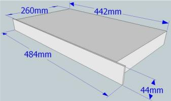
Figure 1: IGC5 dimensions. Allow 50mm (2") at rear for earth stud and connectors
