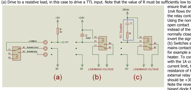
ensure that at least 1mA flows through the relay contacts. Using the normally open contact instead of the normally closed to invert the signal. (b) Switches a mains contactor, for example a heater. To comply with the 1A contact current limit, the resistance of the external relay coil should be  $>30\Omega$ . Note the reverse biased diode MUST
